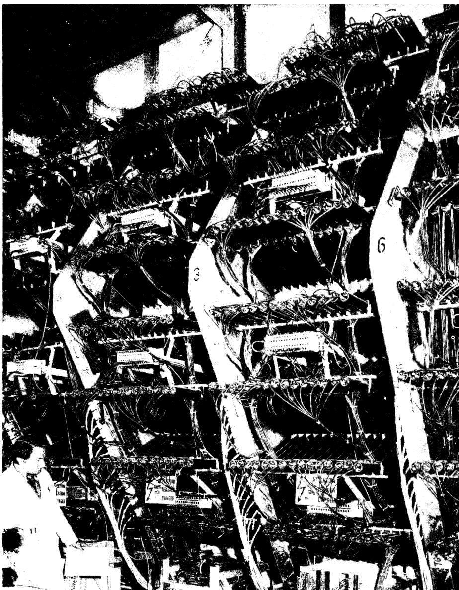
Modules of the CERN / Dortmund / Heidelberg / Saclay high energy neutrino experiment (WA1) at the SPS. Similar modules could be used in a new experiment using a low energy neutrino beam to look for signs of neutrino oscillations.
